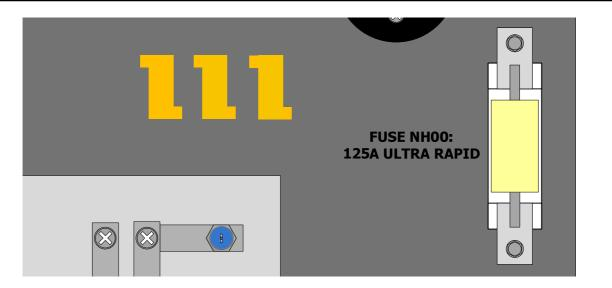
To prevent consequential damage in case of an AVR or generator failure, the AVR supply is fused by a 125A ultra rapid fuse.
