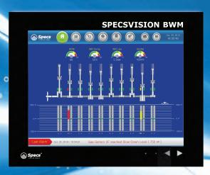
SPECSVISION-BWM is a useful tool for predicting bearing wear in 2-stroke engine before it becomes critical condition and the system provides early alarm or slowdown signal if unexpected problem occurs at the crank-train bearings comprised of crosshead, crank and main bearings during engine operation.
